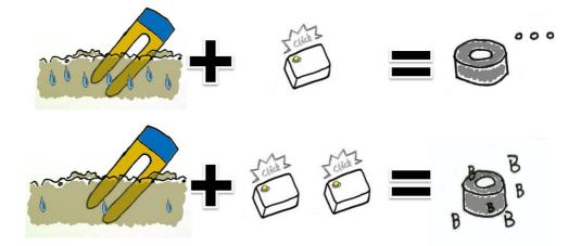
In our first example above, submerge the sensor in moist soil and single click the yellow "set" button on MilCandy to tell the buzzer to remain silent.
