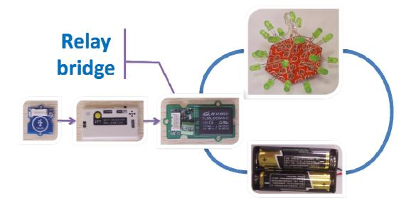
Signals from the input sensor are passed down to the relay through MilCandy. Once the relay receives the message, it translates it into either connected or disconnected in the second circuit.
