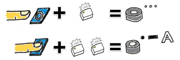
In our first example above, do not press the touch sensor and single click the yellow "set" button on MilCandy to tell the buzzer to remain silent.
