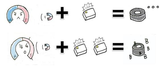
In this scenario, the magnetic sensor, MilCandy, and buzzer are assembled and attached to a door. A magnet is placed on the wall which the door opens into.
