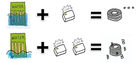
In our first example above, submerge the sensor and single click the yellow "set" button on MilCandy to tell the buzzer to remain silent.
