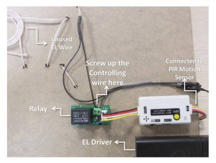
Now it's time to set the logic for MilCandy. When the motion sensor is not activated, click the yellow "set" button on MilCandy. As a person walks by the motion sensor, double click the yellow "set" button on MilCandy to activate the EL wire image.
